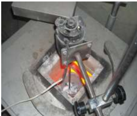
Fig 2.1 Stir casting furnace
