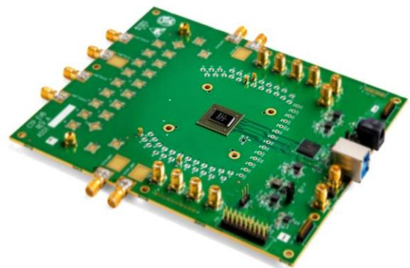
**Fig-2:** Vayyar RF 3D Imaging Sensor
