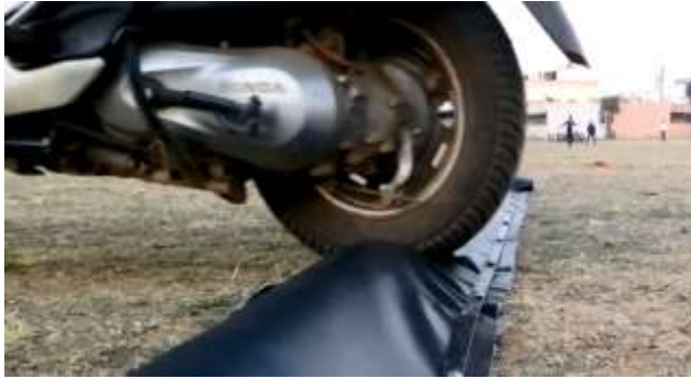
Fig: Deformation of breaker
