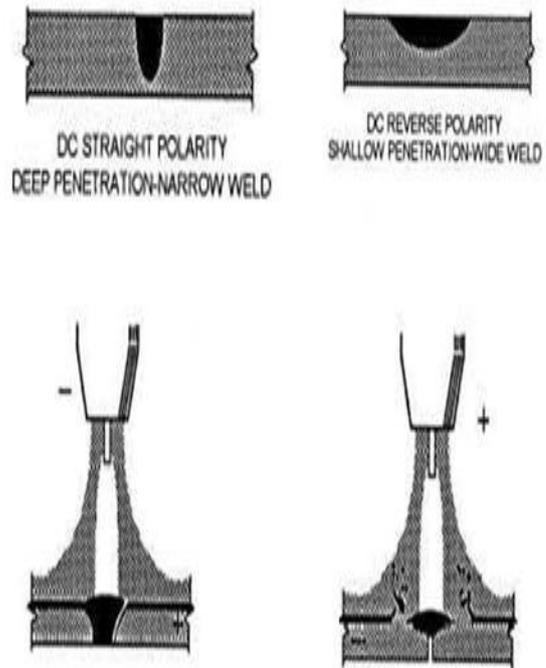
Figure.2 DCSP TIG and DCRP TIG weld formation
