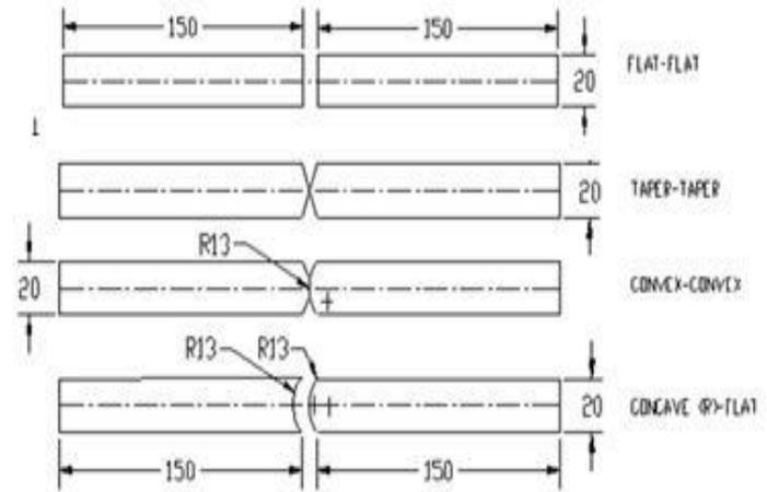
Figure 3.21: Interface geometry combinations for FW
