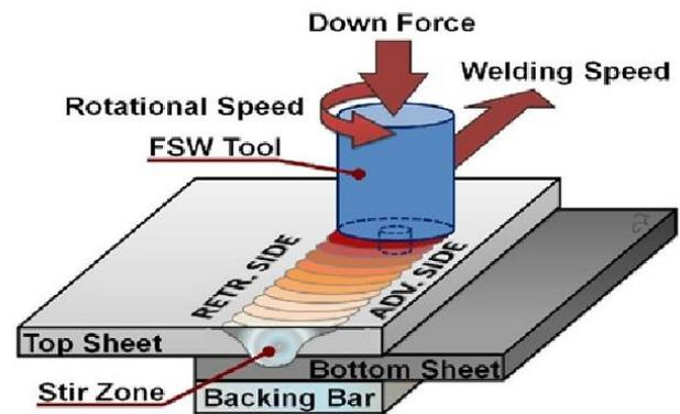
Figure 1.1: Schematic drawing of friction stir welding
