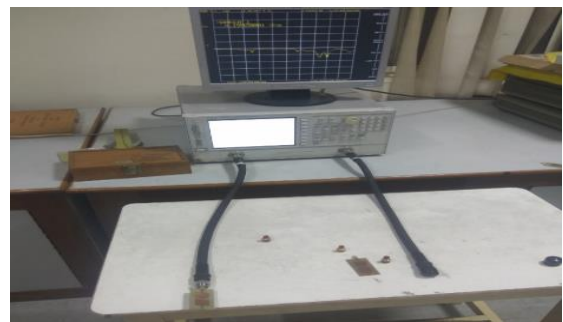
Fig-7: Antenna testing using Network analyzer
