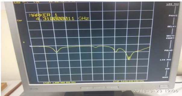
Fig-8: Return loss for linear polarization
