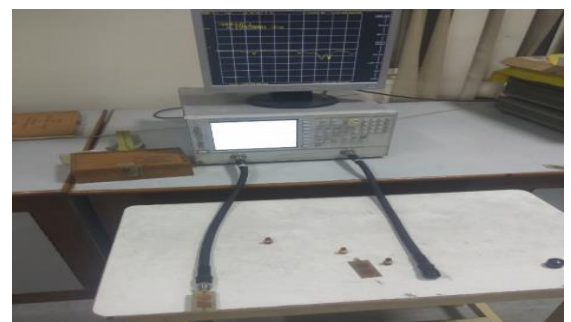
Fig-7: Antenna testing using Network analyzer
