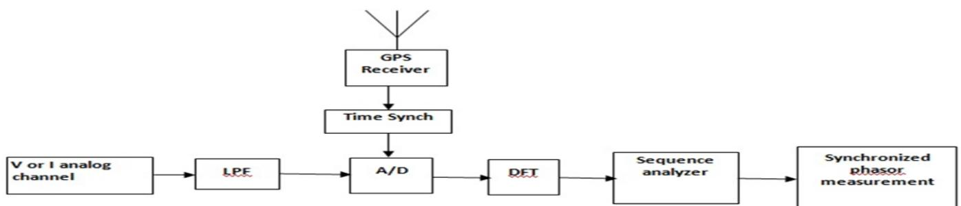
Fig -1: Control System in WAMS
