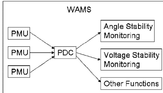
Fig-3: Typical PDC in WAMS
