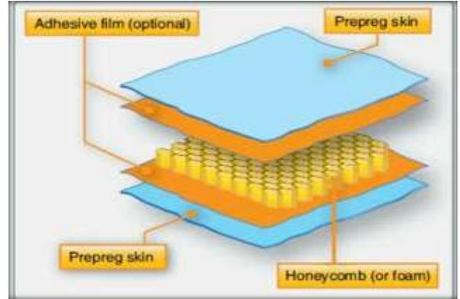
Fig.2: Sandwich structure
