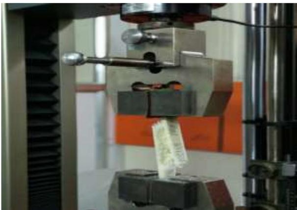
Figure.8: Tensile Testing of Specimen
