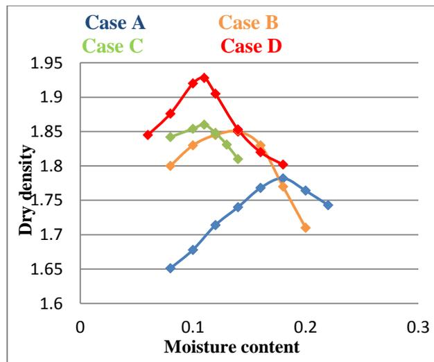
Fig.5: Modified proctor test comparison graph
