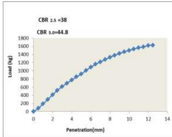
Fig.12: CBR Test Result, Case C (Un-soaked)
