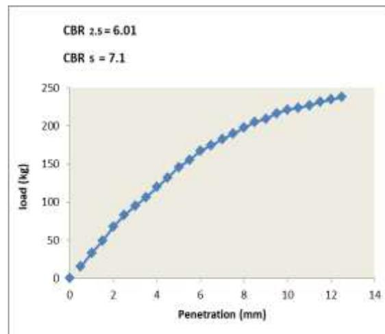
Fig.13: CBR Test Result, Case C (4 days of soaking)
