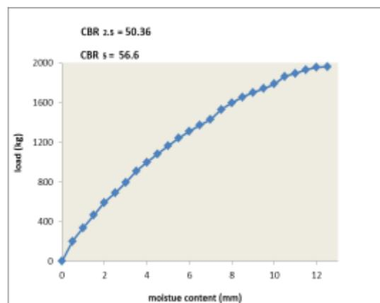
Fig.14: CBR Test Result, Case D (Un-soaked)
