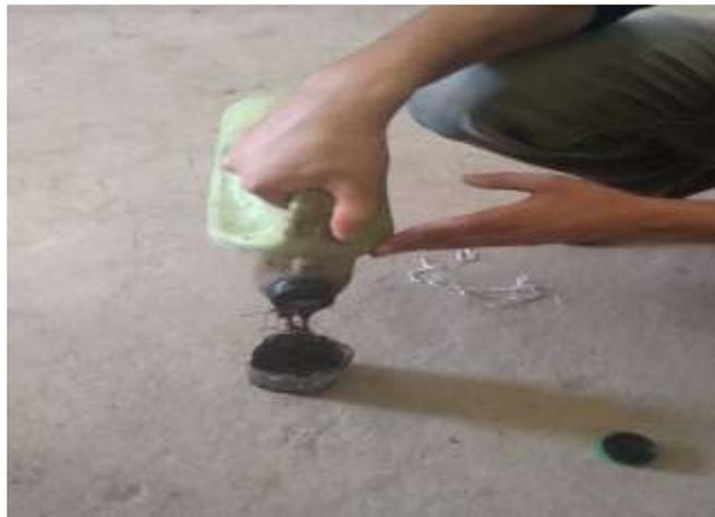
Fig.2: Bitumen emulsion sample
