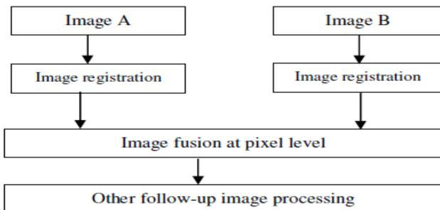
Figure 1: Pixel level fusion
