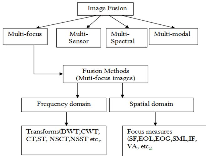
Fig.4. Methods used in multi-focus image fusion
