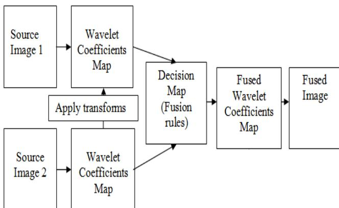
Fig.5. Frequency domain image fusion process
