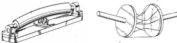
Fig -5: Swash Plate engine
