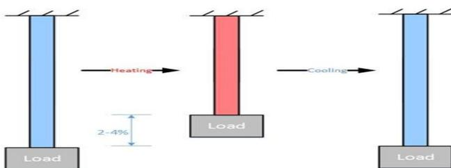
**Fig. -1:** Work cycle from heating and cooling Shape Memory Alloy<sup>[4]</sup>
