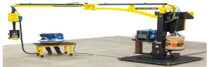
Fig.1: Normal articulating boom used for handling a welding machine [7]
