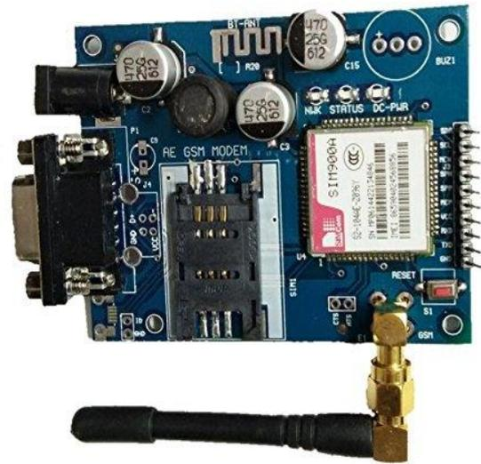
Figure 7: SIM900A GSM/GPRS module
