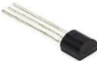
Figure 6: LM35 temperature sensor
