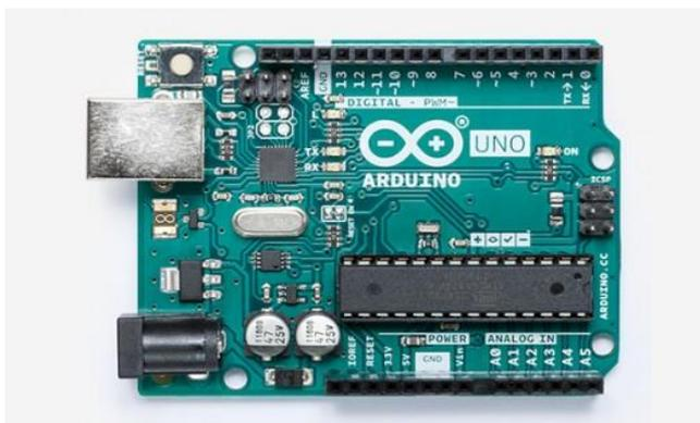
Figure 1: Arduino Uno microcontroller
