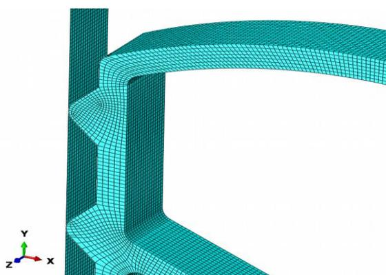
Fig-4: FEM of Bridge joint seal with loads and boundary condition
