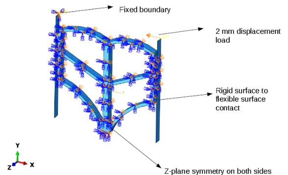
**Fig-3:** Fine mesh of bridge joint seal enlarged
