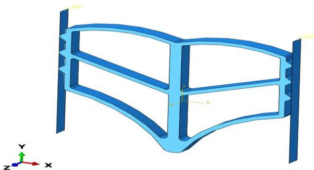
**Fig -1:** Cross section 3D model of the seal
