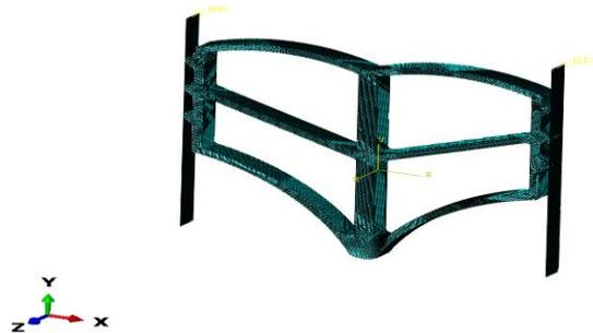
**Fig-2:** Finite element models of bridge joint seal
