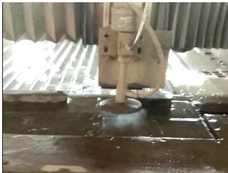
Fig -2: CNC Water jet Cutting of plate.
