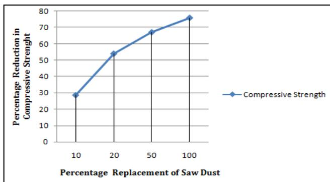
Figure 2: Percentage Reduction in Compressive Strength
