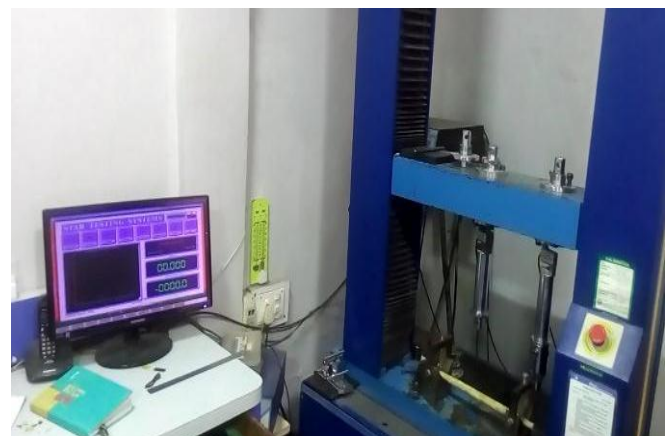
Fig-20: Testing on Universal Testing Machine
