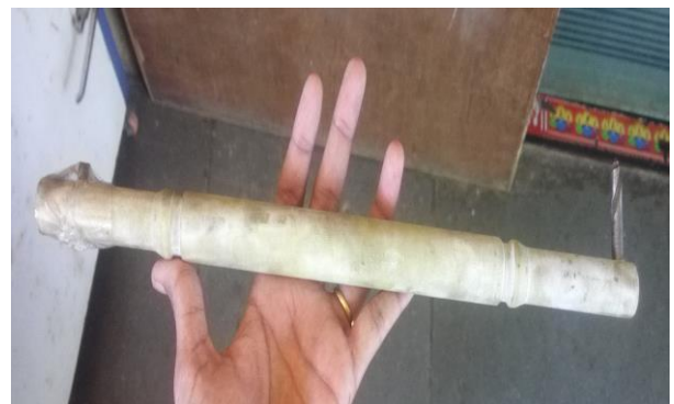
Fig- 19: Fabricated glass fiber reinforced drive shaft
