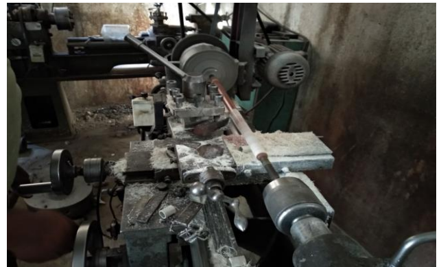
Fig-18: Manufacturing of glass fiber reinforced drive shaft
