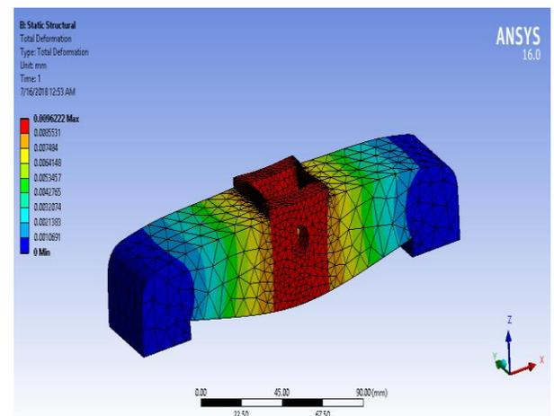
Fig -3.2: Total deformation in clamp
