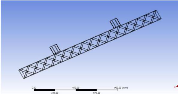
**Fig1.2:** Wireframe view of side impact structure
