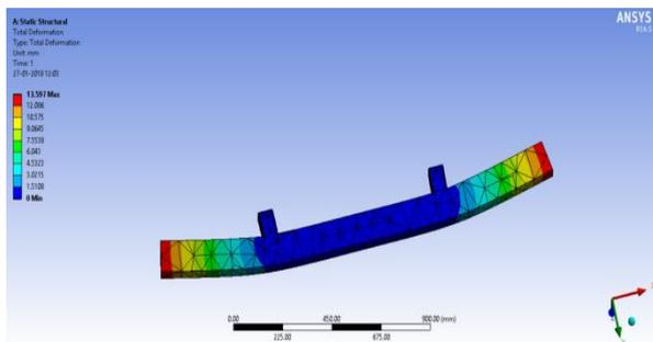
**Fig3.3:** Total deformation for Ti alloy on side impact
