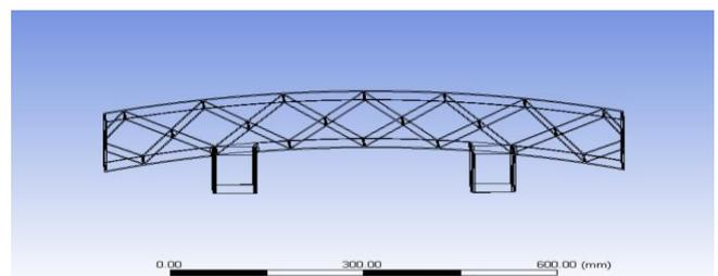
Fig1.1: Wireframe view of front impact structure
