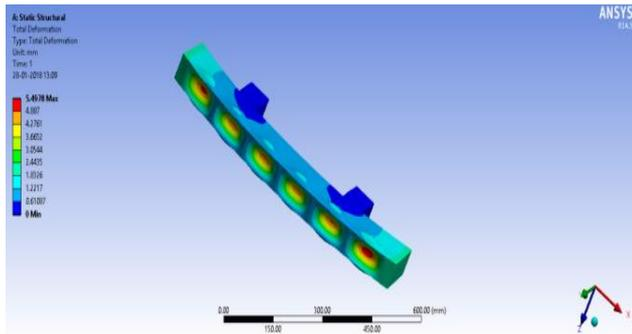
**Fig3.1:** Total deformation for Ti alloy on front impact
