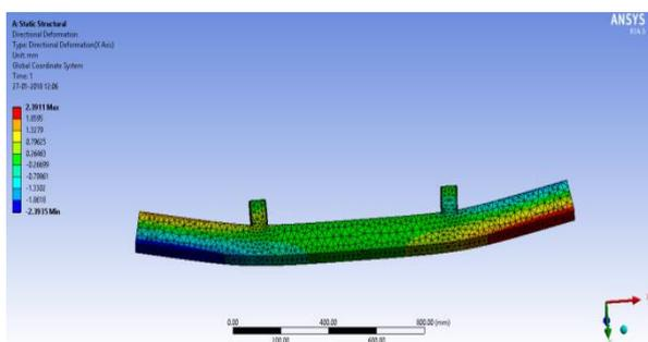
**Fig3.4:** Directional deformation for Ti alloy on side impact
