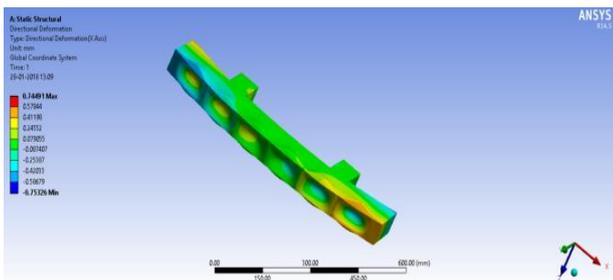
**Fig3.2:** Directional deformation for Ti alloy on front impact
