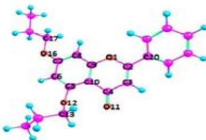
Figure.3: Optimized (BP86/TZVP) geometry for the compound 5, 7-diethoxy-2-phenyl benzopyran 4H-one
