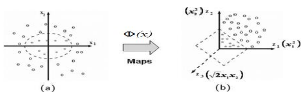
Fig -2: Example for SVM Kernel Function \Phi(x) Maps 2-Dimensional Input Space to Higher 3-Dimensional Feature Space. (a) Nonlinear Problem. (b) Linear Problem.
