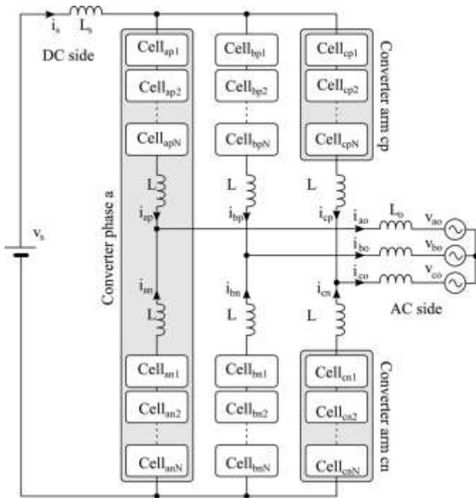
**Fig2.** DC/Three-phase modular multilevel converter circuit topology
