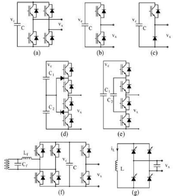
**Fig. 3.** Power cell topologies. (a) Full-bridge. (b) Half-bridge. (c) Unidirectional cell. (d) Multilevel NPC cell.
