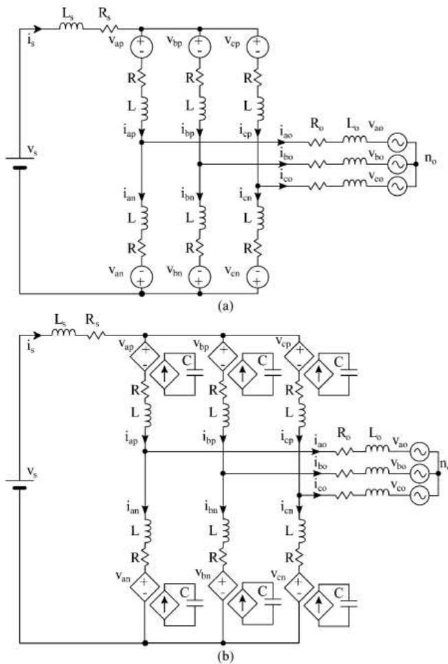
**Fig. 4.** Models of the M<sup>2</sup>C. (a) Considering the arms as voltage sources. (b) Considering switching effects and capacitor dynamics.
