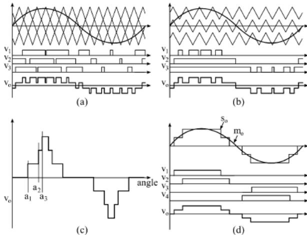
Fig. 5. Modulation techniques. (a) Phase shifted PWM.
