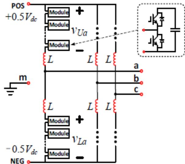
Fig. 1. The schematic of the modular multilevel converter ( $M^2C$ )
