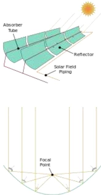
Fig -2: A diagram of a parabolic trough solar collector
