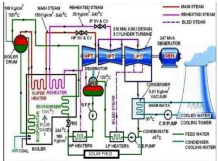
Fig -1: Solar Thermal Power Plant Using PTC
