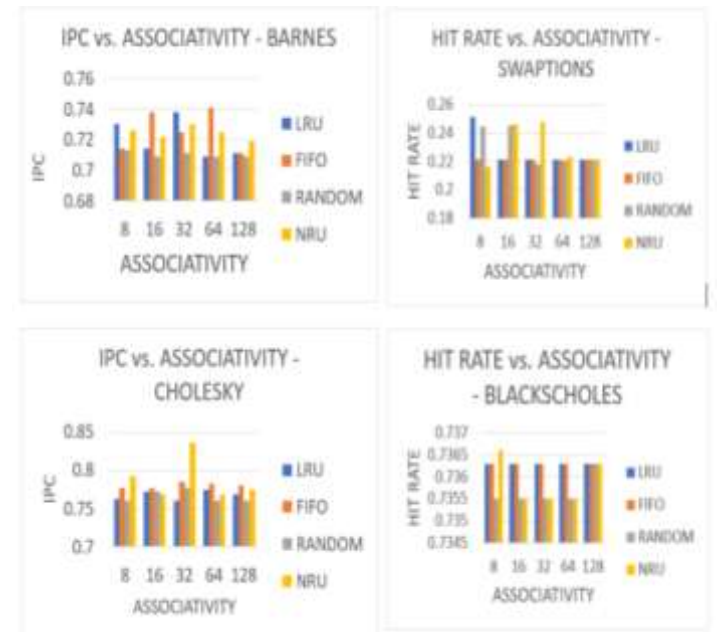
Fig -1: IPC/Hit Rate vs. Associativity for different benchmarks, for LRU, FIFO, NRU and RANDOM replacement policies.
