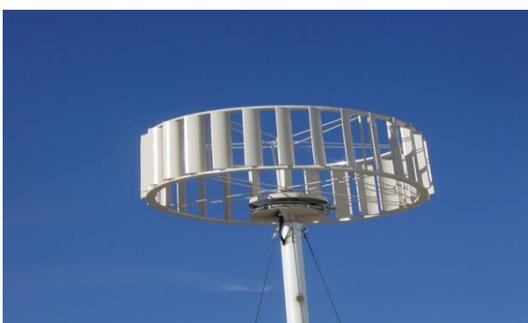
Figure 2: Vertical Axis Wind Turbine
