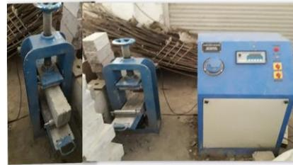
Figure 4.4: Flexural testing machine at beam size (700\*150\*150 mm<sup>3</sup>).
