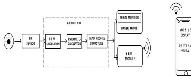
Fig. 1 : Block-diagram of the UBI
