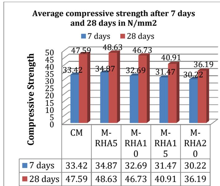
Chart-1: Effect of Rice Husk Ash on Compressive strength of concrete
