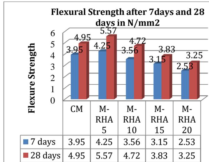
**Chart-3:** Effect of Rice Husk Ash on flexural strength of concrete
