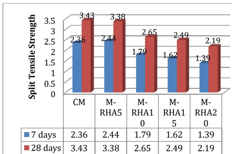
Chart-2: Effect of Rice Husk Ash on split tensile strength of concrete
