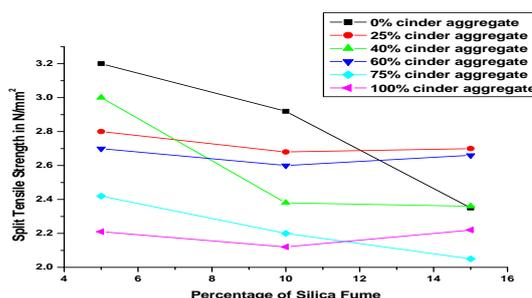
**Fig-3:** Split Tensile strength with different percentages of cinder aggregate with different percentages of fly ash
