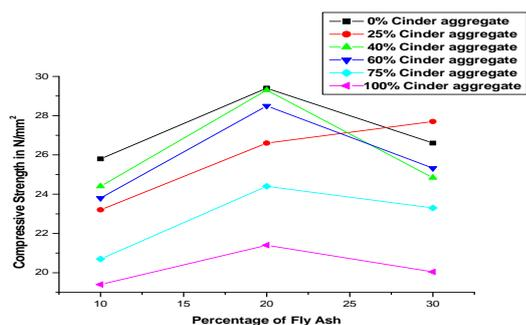
**Fig-2:** Compressive strength with different percentages of cinder aggregate with different percentages of fly ash
