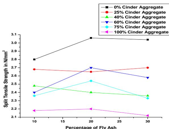
**Fig-4:** Split Tensile strength with different percentages of cinder aggregate with different percentages of fly ash
