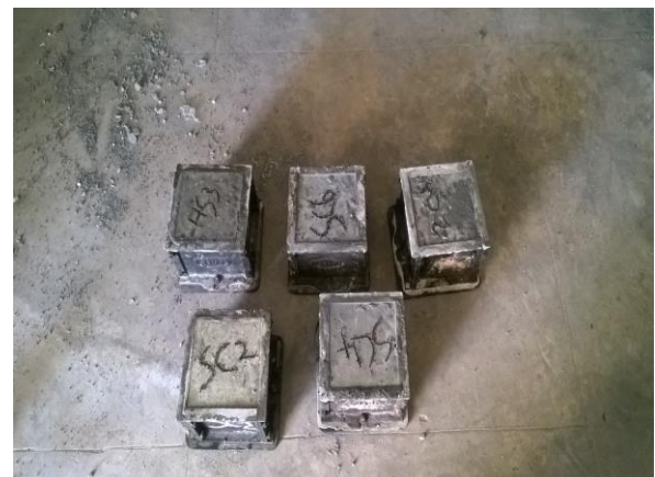
Fig 3 – Casting of concrete specimens
