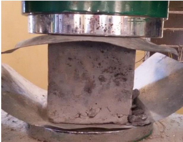
Fig 4 - compression Testing of Concrete cube specimen
