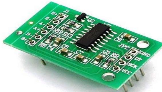
Fig. 5: Diagram of the Hx711 Load Cell amplifier Module
