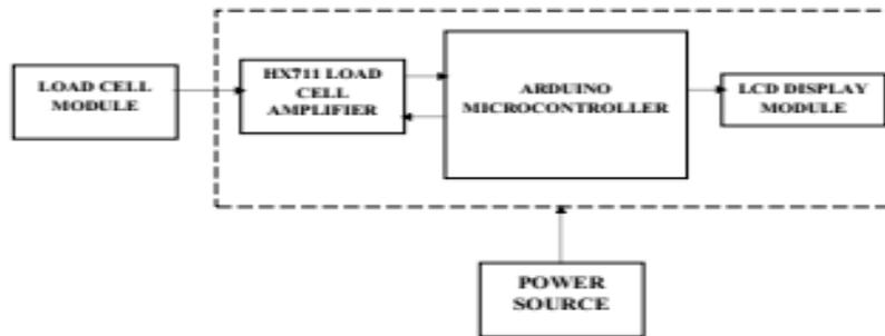
Fig. 1: System Architecture
