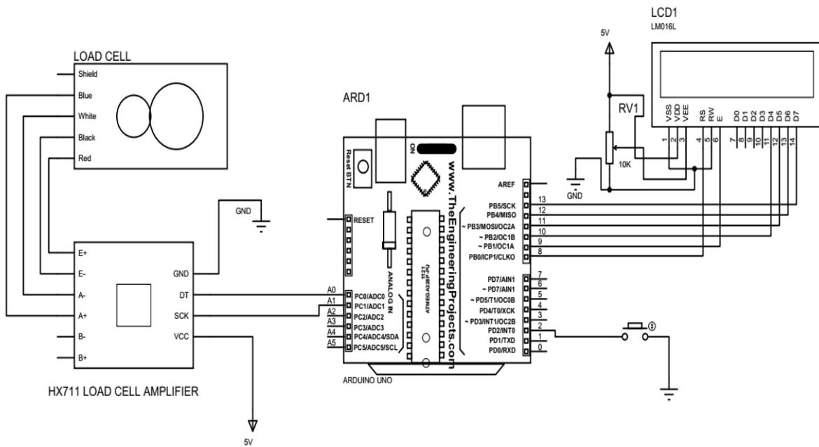
Fig. 3: Circuit diagram for the developed system
