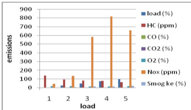
Chart- 2: Load vs Emission Analysis for pure diesel
