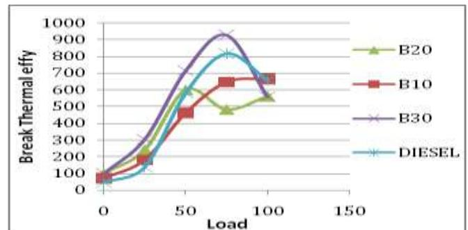
Chart- 5: Comparison of Load Vs Brake thermal efficiency for different blends of algae oil.
