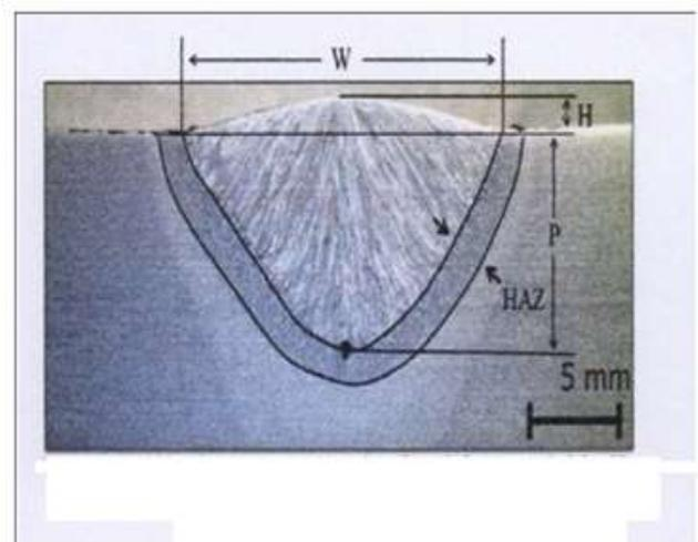
Figure 4 H-Reinforcement, p-penetration, HAZ-Heat affected zone-width
