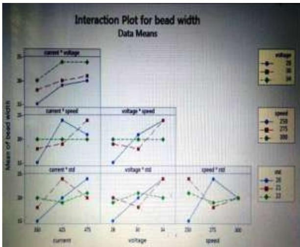
Figure 7 Interaction plot for bead width
