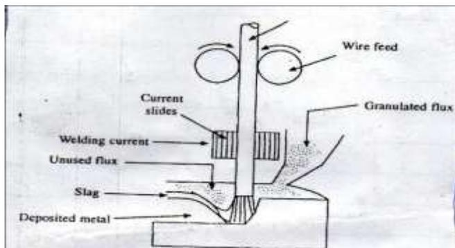
Figure 2 Schematic Dig. Of Saw Machine.
