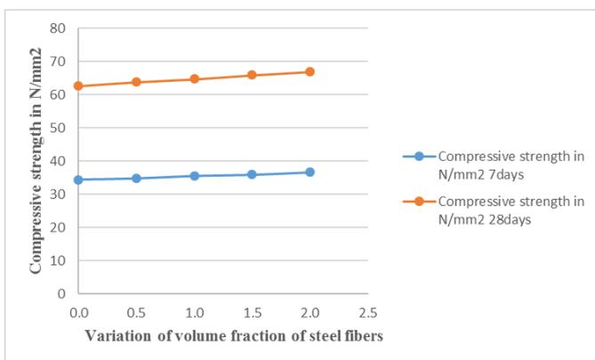
Figure 3: Variation of compressive strength for percentage variation of volume fraction of steel fibers for M-Sand optimized SCC
