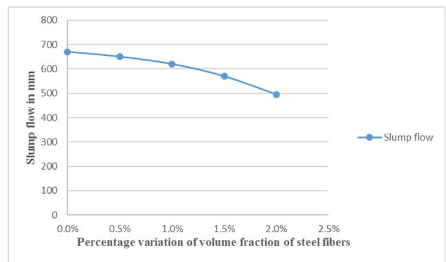
Figure 1: Slump flow for percentage variation of volume fraction of steel fibers
