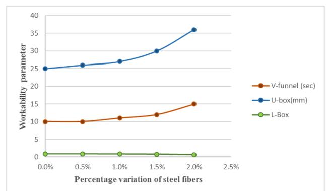
Figure 2: Workability parameter (L-Box, V-Funnel, and U-Box) for percentage variation of steel fibers
