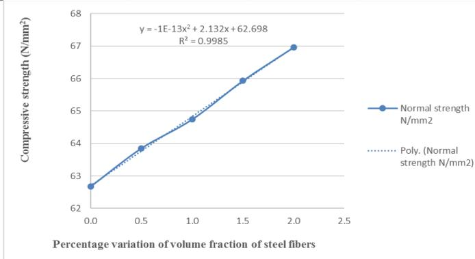
Figure 5: Best fit curve for compressive strength
