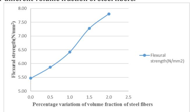
Figure 4: Variation of flexural strength due to percentage variation of steel fibers for M-Sand optimized SCC
