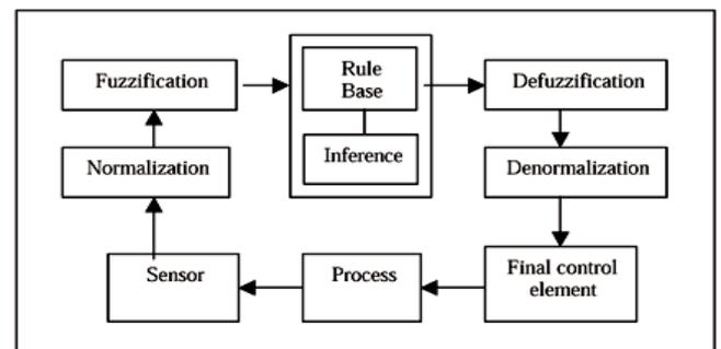
Fig -4: Block diagram of Fuzzy Logic controller
