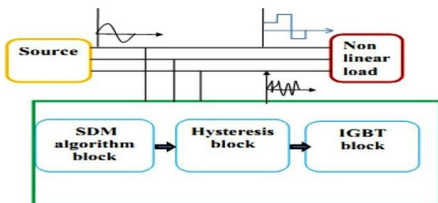
Fig -3: SDM filter block [22]
