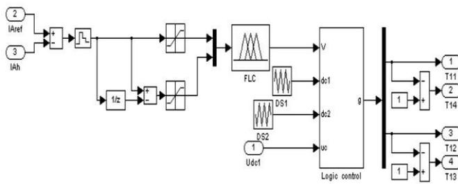
Fig-6: Three-level inverter switching signal generation
