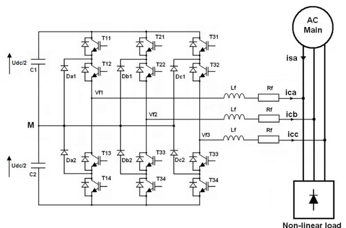
**Fig -1:** Three level shunt active filter
