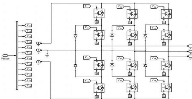
Fig -2: Three-level NPC inverter
