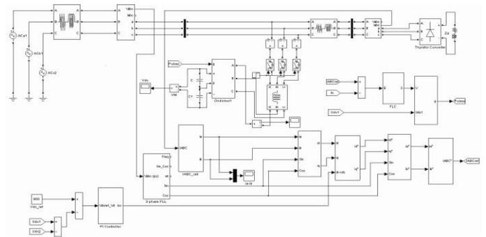
Fig-7: Three-level shunt active filter based on fuzzy current controller
