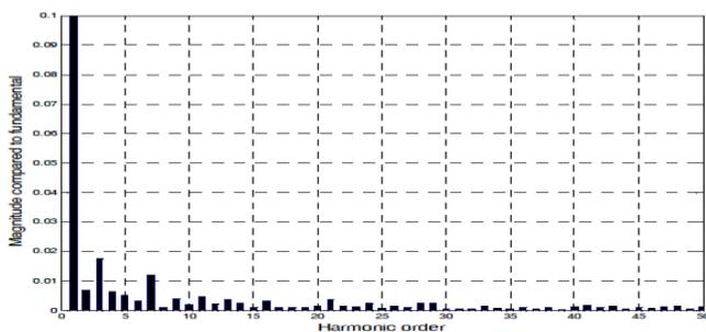
Fig -13: Source current spectrum with APF using fuzzy controller (THD 1.27%)
