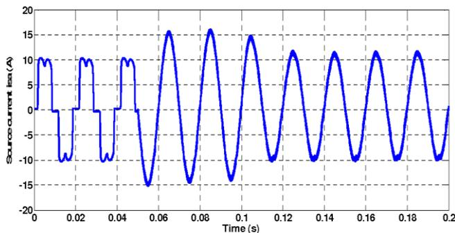
Fig -12: Source current before and after compensation using Fuzzy controller
