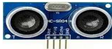
Fig 1.7: Ultrasonic Sensor HC SR-04
