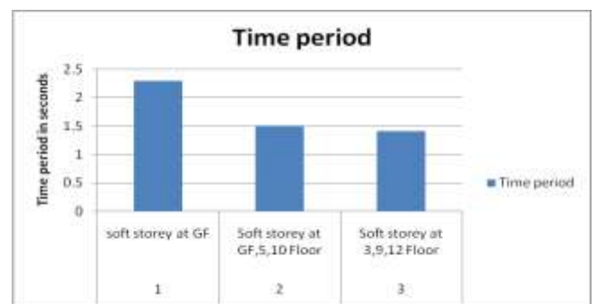
Fig 8: Graph of time period of models with shear wall for seismic zone III & V.
