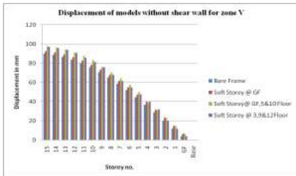
Fig 5: Graph of displacement of model without shear wall for Zone V in x direction.
