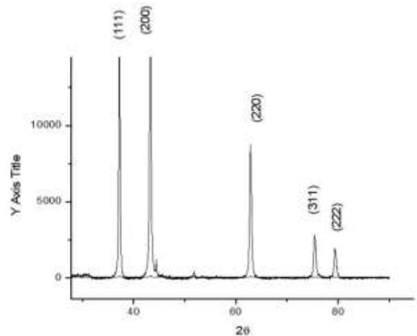
Fig. 9 XRD spectra of neodymium doped nickel oxide
