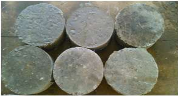
Figure 16 Test Specimen with 1 % of Crimped Fiber
