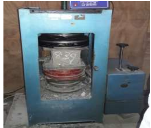
Figure 9 Compressive Strength Testing
