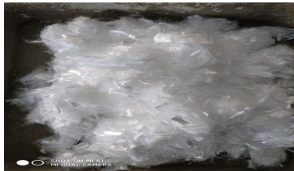
Fig 1: Sample of polypropylene fibre
