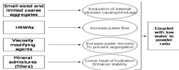
Fig -1: Principles of SCC Mixture Design
