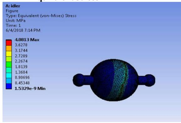
**Fig. 8:** Equivalent stress
