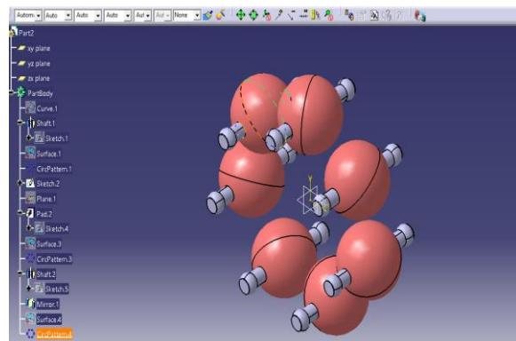
**Fig. 5:** 3D model of spherical balls
