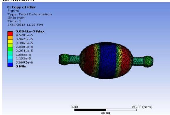
**Fig. 9:** total deformation under ideal running condition
