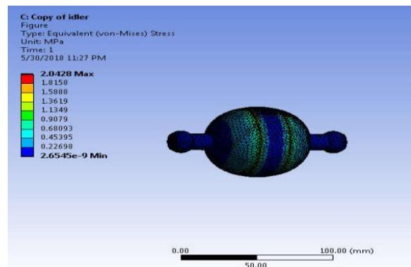
**Fig. 10:** Fixed equivalent stress.
