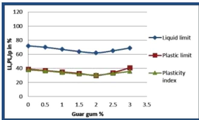
**Figure 4.1: Plasticity Characteristics of guar gum Admixed Soil.**
