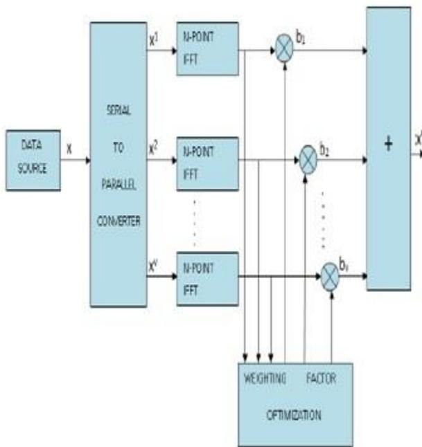
Figure 3: Block Diagram of PTS
