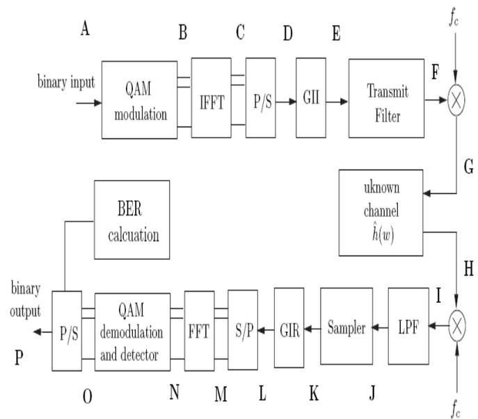
Figure 1: OFDM block diagram.
