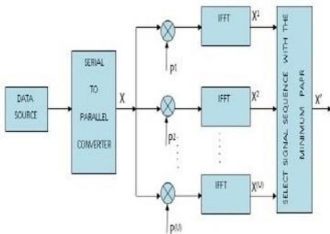
**Figure 2: Block Diagram of SLM**
