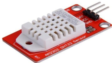
Fig-2: DHT 22 temperature and humidity sensor
