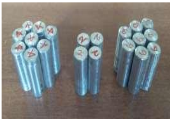
Fig 2. Specimen Pin For Wear Test.
