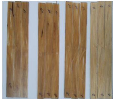
Figure-2: Tensile Test Specimens.
