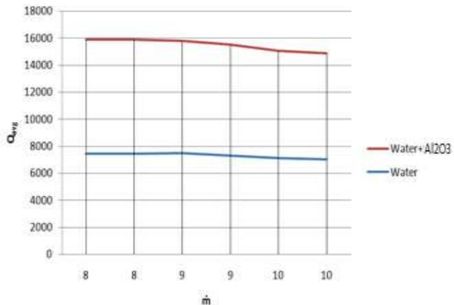
From the above graph we concluded that: From graph we see as we decreases the mass flow rate, there is average heat transfer rate of the nanofluid increases. In the graph shows average heat transfer of the nanofluid is greater than water.
