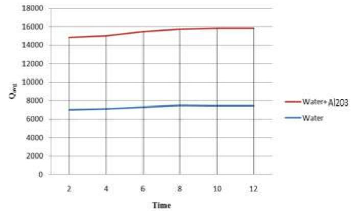
From the above graph we concluded that: With increases the time the average heat transfer rate also increases. Nanofluid gives better heat transfer than water.
