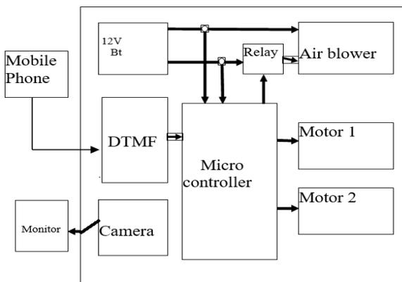
Fig -1: Block diagram of a duct cleaning vehicle
