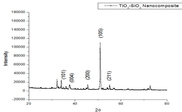
Fig.3 (b) X-Ray Diffractogram of TiO<sub>2</sub>-SiO<sub>2</sub> Nanocomposite
