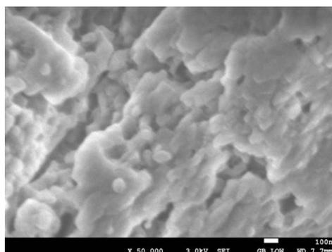
Fig.4(a) FESEM image of TiO<sub>2</sub> nanoparticle
