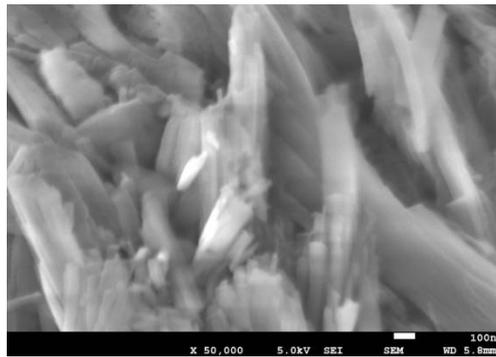
Fig.4(b) FESEM image of TiO<sub>2</sub>-SiO<sub>2</sub> nanoparticle
