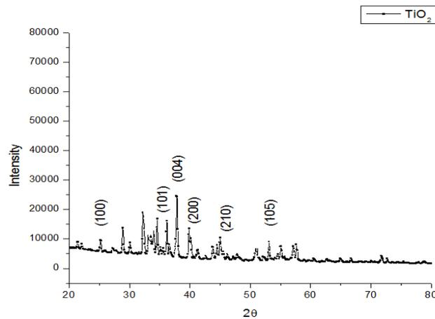
Fig.3(a) X-Ray Diffractogram of TiO<sub>2</sub>
