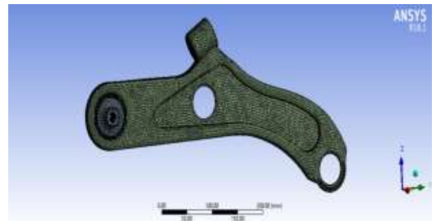
Figure 2 Meshed model of control arm
