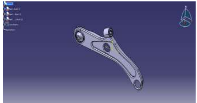
Figure 1 CAD Model of control arm
